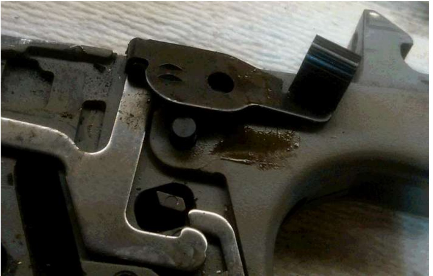
This shows the Manual Safety removed from the Hammer Pin.
